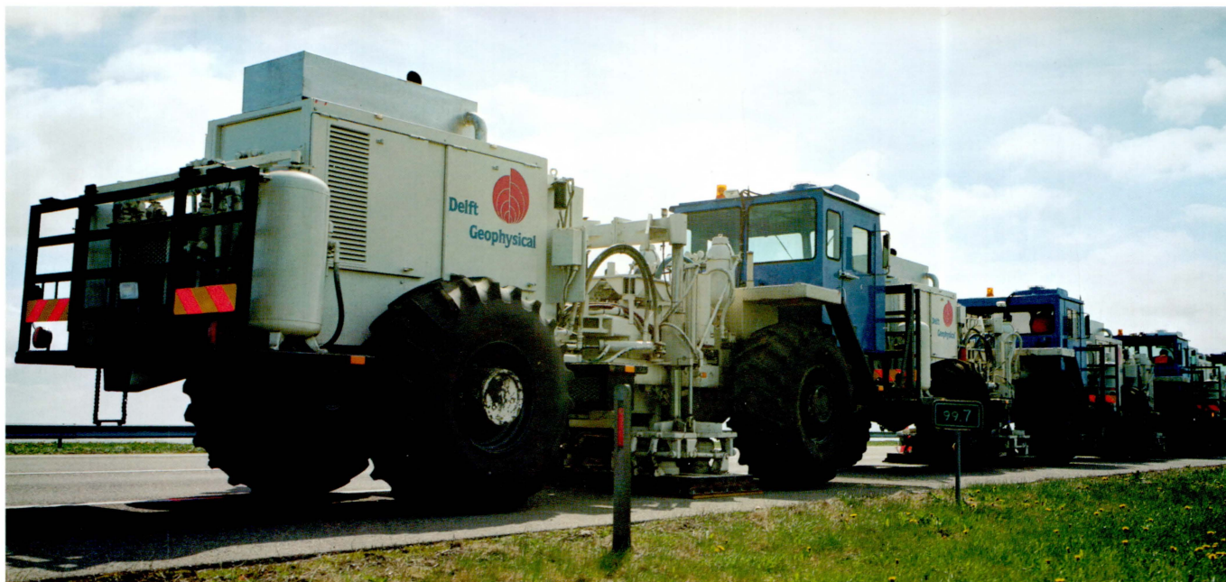
Vibrator equipment generates acoustic signals for seismic investigations.
